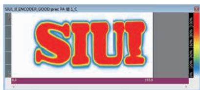
C Scan In-Amplitude, showing echo amplitude
