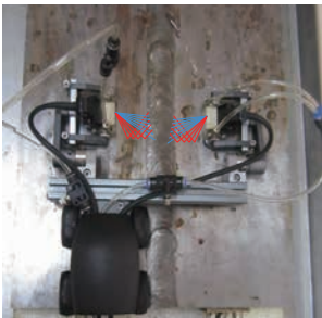
Dual-side Butt Weld Inspection
